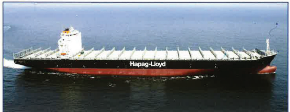
The photograph shows MV "Savannah Express", a newbuilding which has come under our Crew-management from Messrs Norddeutsche Reederei H. Schuldt. The vessel which is chartered by Hapag-Lloyd is one of the biggest containerships in the market and has capacity 8,400 TEU. She is flying the German flag, is 332.40 m long, 43.30 m wide and capable of steaming at 25.40 Kts.
