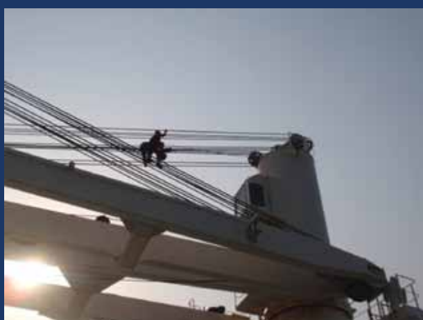
1 Greasing Wire During drifting in gulf of guinea on MV United Milos by Chief Officer Marius Ovidiu Ionascu
